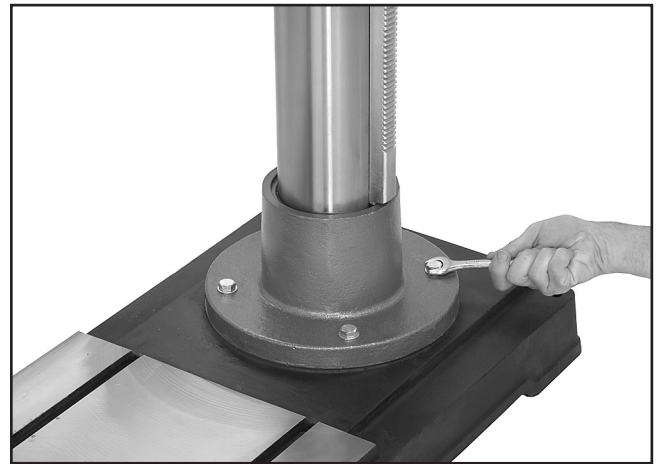
Figure 6. Assembled column and base.
